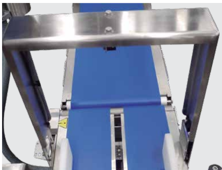
> Vertical detector on arch
